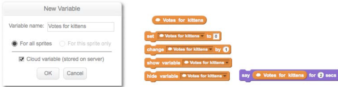
Figure 1-4: Programmer interactions for using Cloud variables in Scratch 2.0 [7]. A variable can be set to be a Cloud variable by selecting the Cloud variable checkbox. A Cloud variable has the same methods/blocks as a normal variable.
