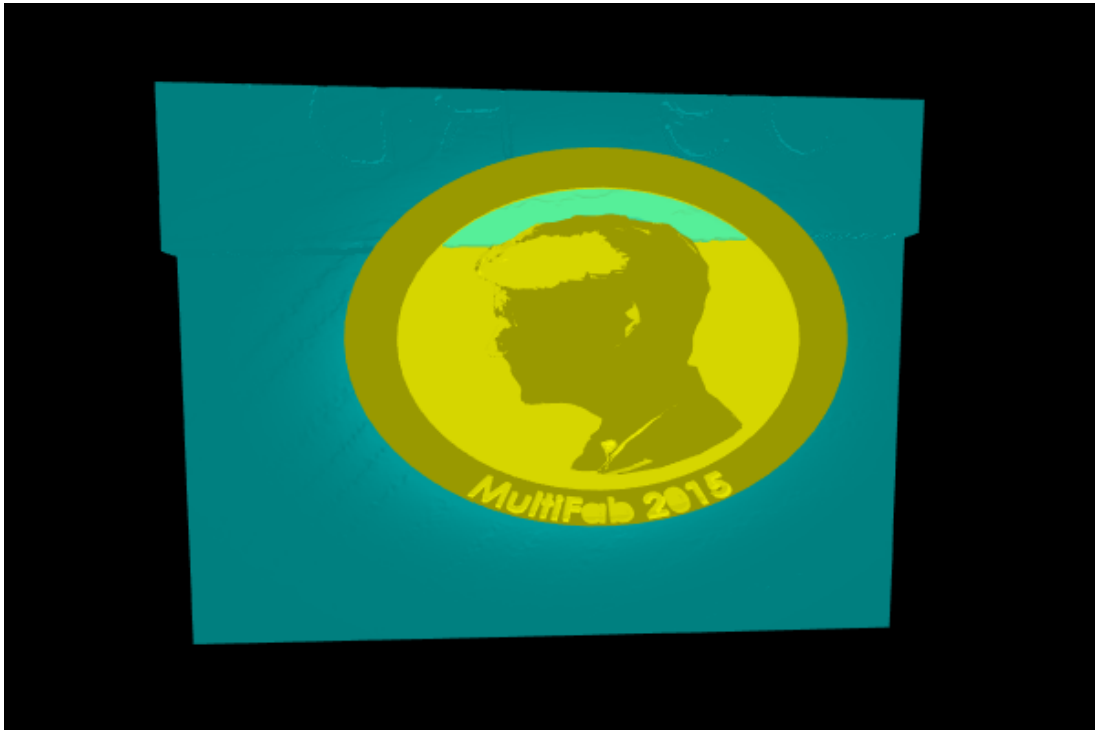
Figure 5-4: An image of the auxiliary positioning. The same depth scan as in figure 5-3 is used. A model of a coin is positioned on top of the depth scan.
