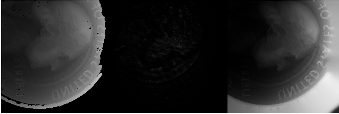
Figure 4-2: An image of a scanned quarter with interpolation. The left image is the depth map with filtered out uncertain points. The center image is the confidence map. The right image is the interpolated depth map.
