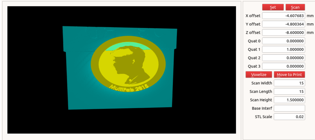
Figure 5-1: An image of the GUI for printing on auxiliary objects. The scan of the auxiliary object is blue and the mesh to be printed is yellow. Controls are on the right.
