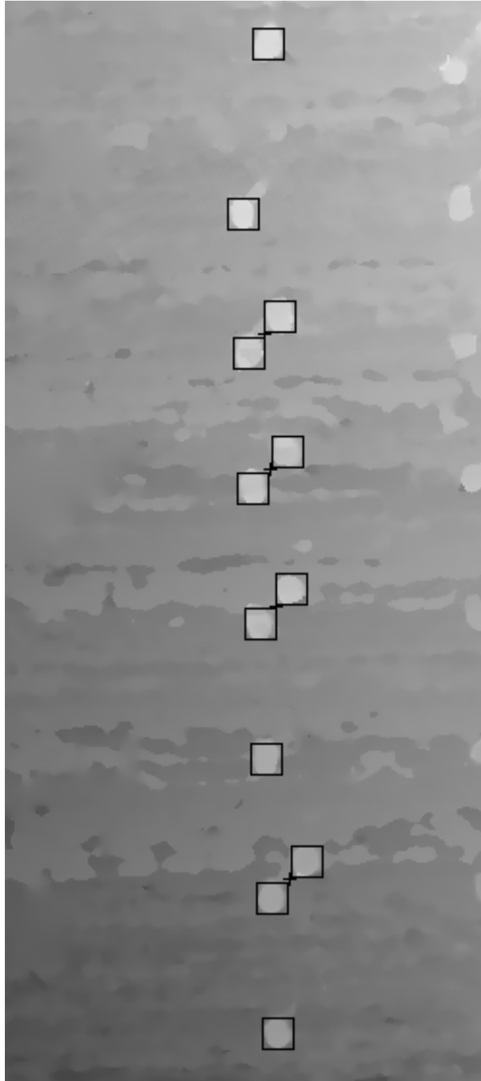
Figure 3-14: An example of cross detection using the depth map. Raised points are outlined by squares. Crosses are marked with a small cross.
