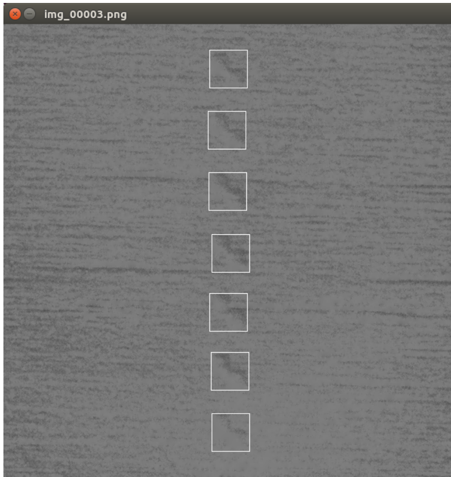
Figure 3-12: The interface for manually labeling crosses for data collection. Clicking on a cross labels the area as a cross.
