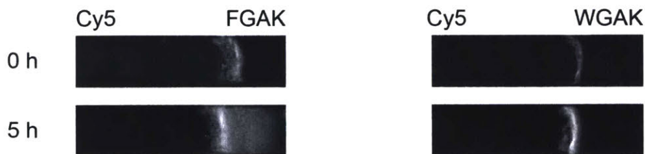
Figure 3-4: Cy5 reporters diffusing into FGAK (left) or WGAK (right) gels over five hours. The five-hour timepoints reveal that Cy5 is able to diffuse significantly further into FGAK than WGAK, suggesting that phenylalanine and tryptophan have different selectivities to the same hydrophobic substrates.
