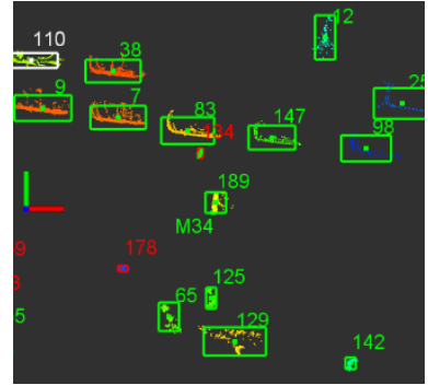
(f) Approximately 0.5 seconds later, the turn is complete. The Velodyne labels persist and the targets are correctly matched.
