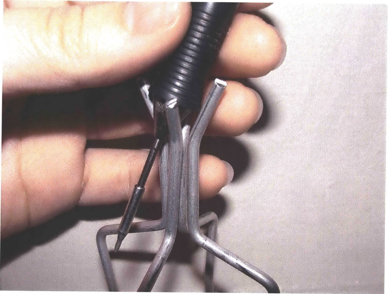
Figure 47: Soldering iron slippage when placed in interlocking supports
