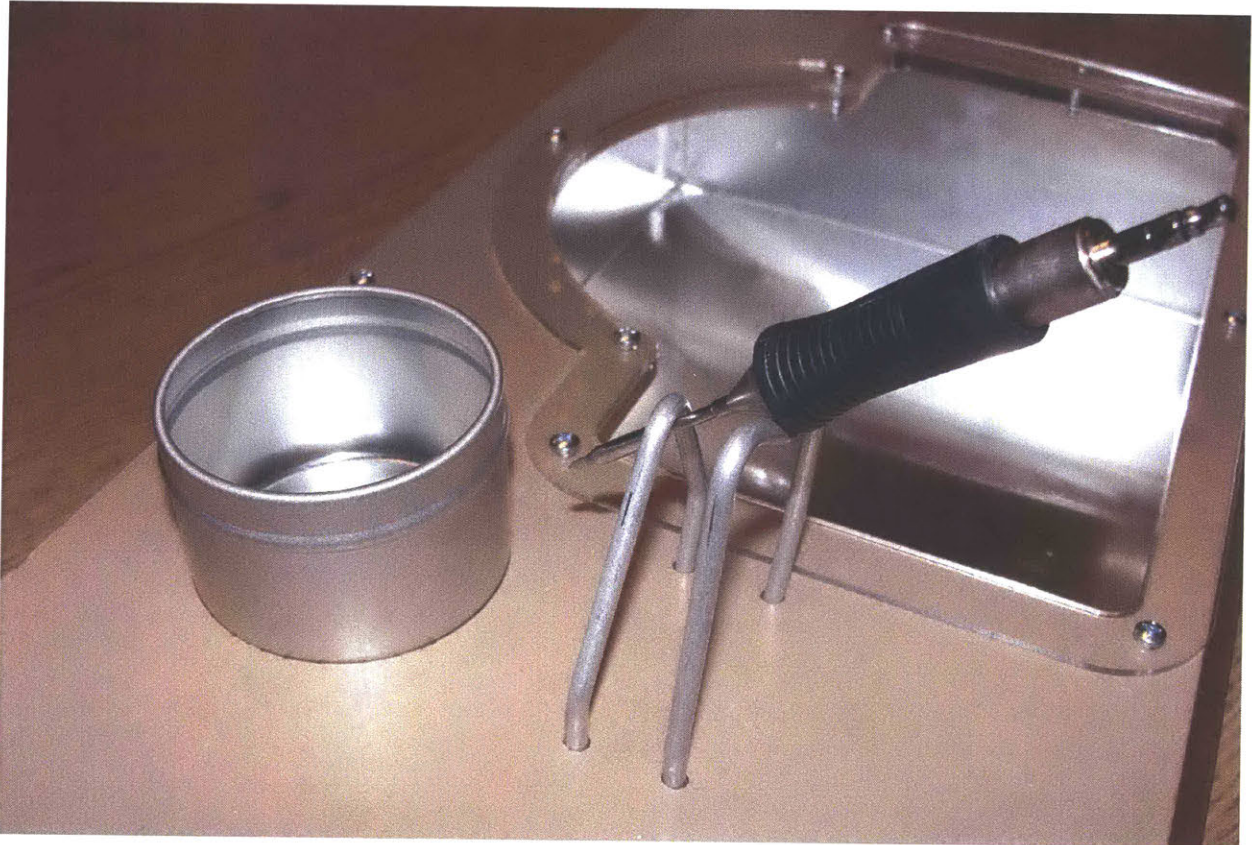
Figure 49: Soldering iron holder and wool pot integrated into the missing panel metal box design
