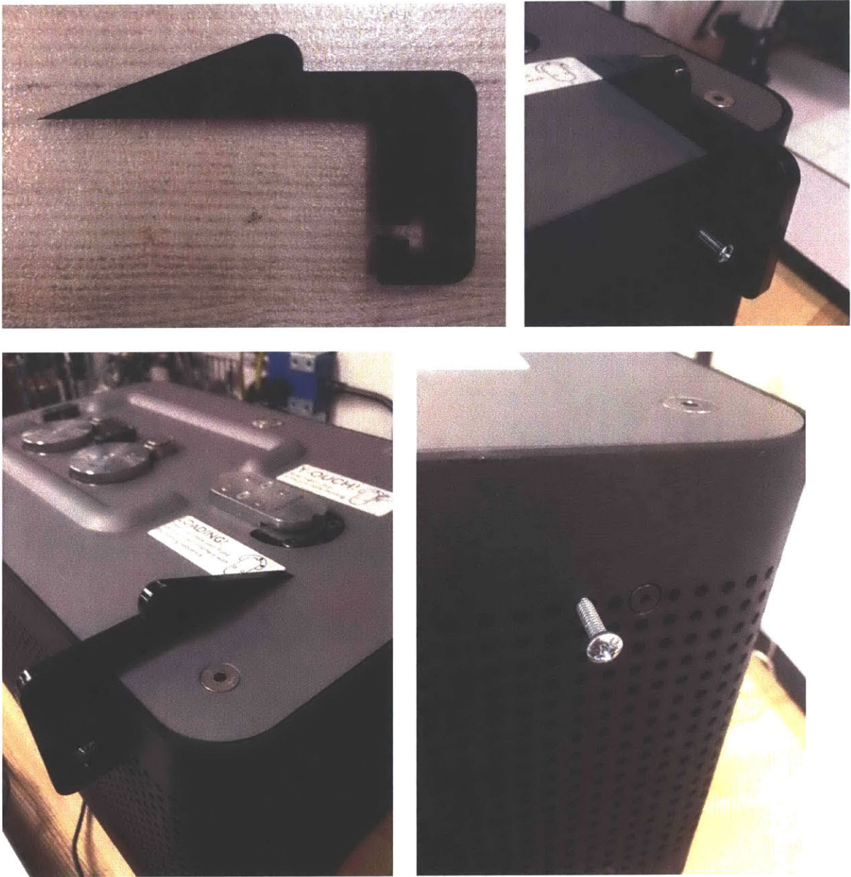
Figure 36: photos showing the laser-cut ramp interfacing with the DiWire
