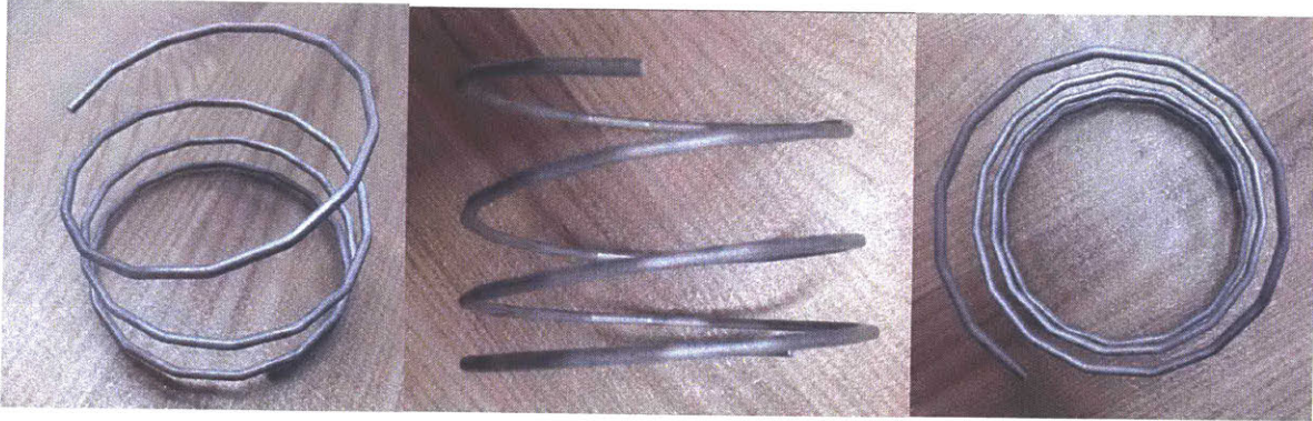
Figure 30: 3 views of a 3 inch diameter spiral bent on the DiWire as a preliminary test
