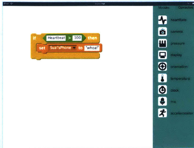
FIGURE 3.13: The “Scratch” interface would use the semi-graphical programming language Scratch to help kids code their device.
