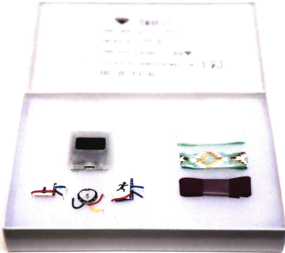
FIGURE 4.18: The complete toolkit with device, sensors, ribbon and guidebook.
