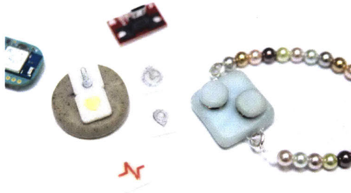
FIGURE 3.10: Snaps were used to imitate electrical connectors between sensor modules and the wearable
