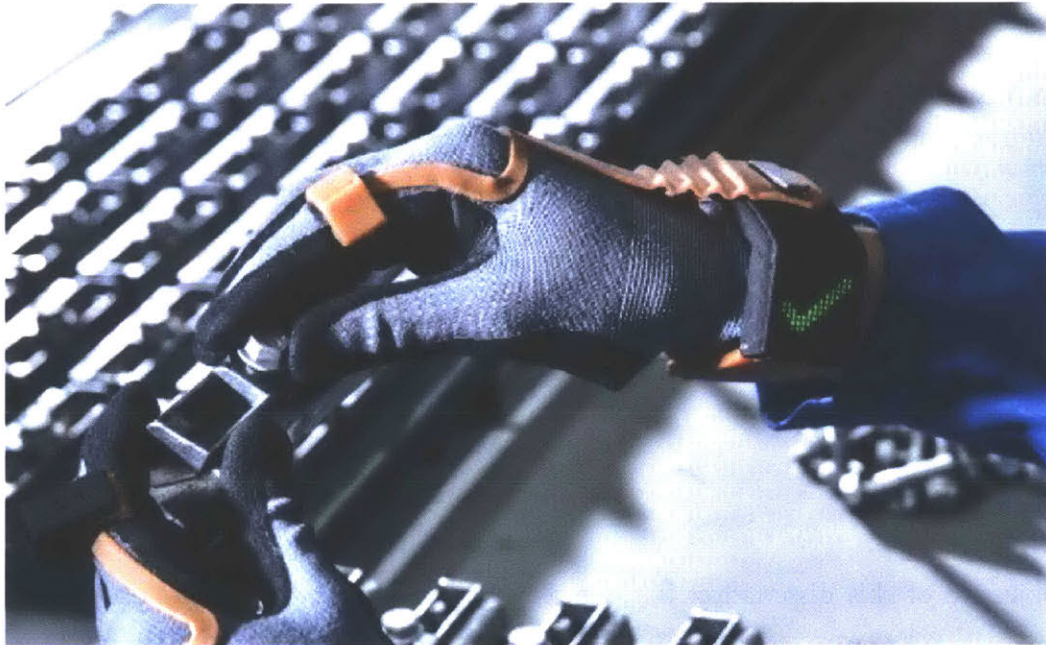
FIGURE 1.7: ProGlove, a wearable for industrial use [33]. It combines an RFID sensor and various other sensors for workflow control.
