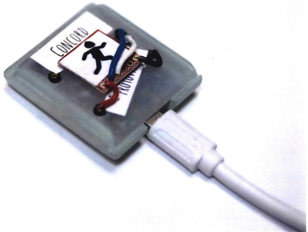
FIGURE 4.4: Sensor with short, extended wires, attached in a compact fashion. Sensors can be connected by plugging wires into header pins. As in electrical standards, the red represents supply voltage and black represents ground. In addition, blue represents SDA, white represents SCL, and yellow (see empty pin on top left) represents the analog sensors signal.
