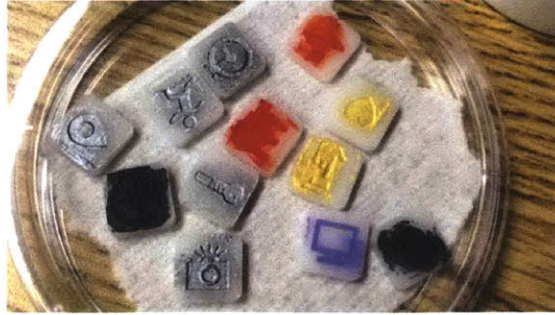
FIGURE 3.9: Acrylic was laser-engraved and painted to imitate specific sensor modules.
