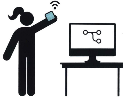
FIGURE 3.5: Concept of the presented design toolkit. A wearable or smart device with (potentially attachable) sensors can be reconfigured wirelessly by using a graphical web application.
