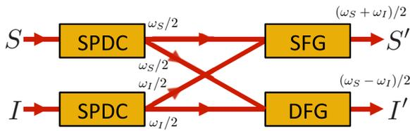
FIG. 4. Notional scheme for approximating the biphoton transform  $\hat{B}_{S'I}$ . SPDC: Single-photon-sensitive spontaneous parametric downconverter with extended phase matching. SFG: Single-photon-sensitive sum-frequency generator. DFG: Single-photon-sensitive difference-frequency generator.
