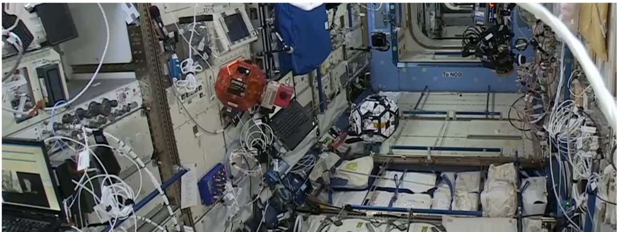
(a) Two SPHERES satellites flying inside the Japanese Experiment Module on the ISS
