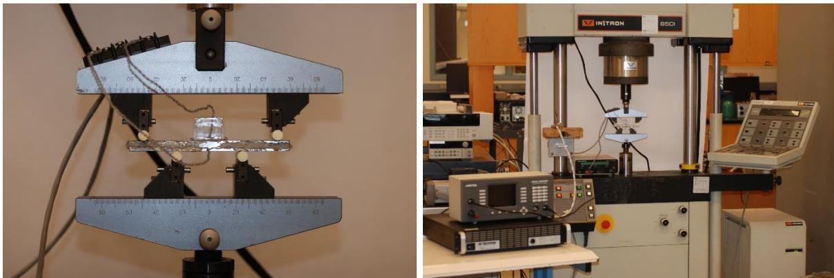
Figure 3-11: System configuration for test in air and aerated NaCl solution at RT.
