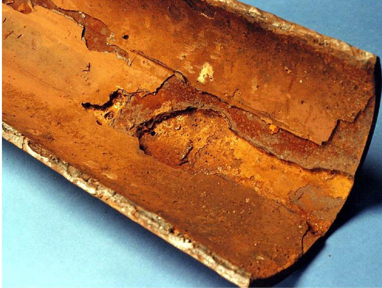
Figure 2-3: A photo of a corroded pipe showing the specific morphology of CO<sub>2</sub> corrosion [37].
