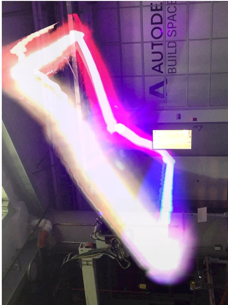
Figure 84: Light painting of ISO 9283 pose repeatability test trajectory
