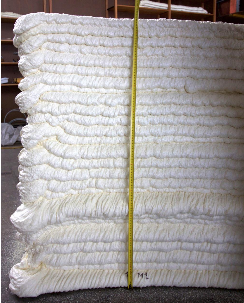
Figure 34: Finished curved wall section layers, with ruler for scale. Image credit: Steven Keating.
