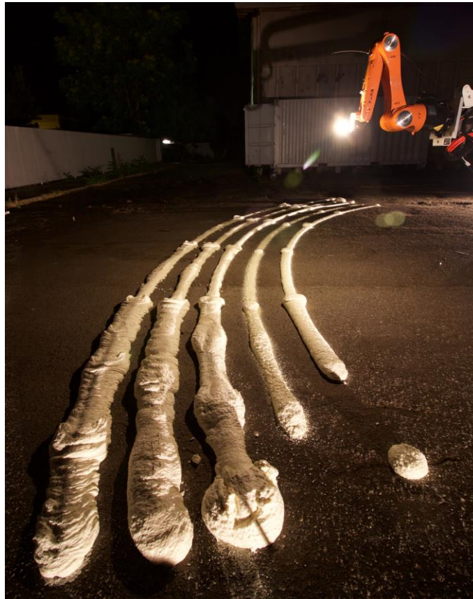
Figure 37: Qualitative determination of optimal feed and flow rate for Print-in-Place process using DCP.
