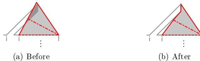
Figure 5-4: Intersection removal. (a) A bridge (red) that intersects with (P, \mathcal{F}) (gray). (b) The offending region is removed.
