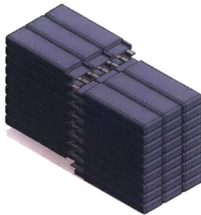
Figure 2-3: Packs of six are wired in series to produce a full battery stack.
