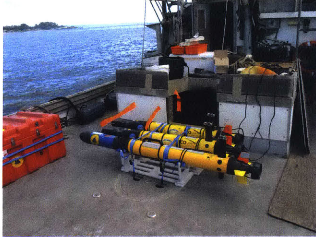
Figure 3-1: OceanServer Iver2 AUVs onboard the R/V Shana Rae . Front to Back: Iver-136, Iver-107, Iver-106. Photo courtesy of Dr. David Frattoni during the KISS Field Project [44] in 2016.
