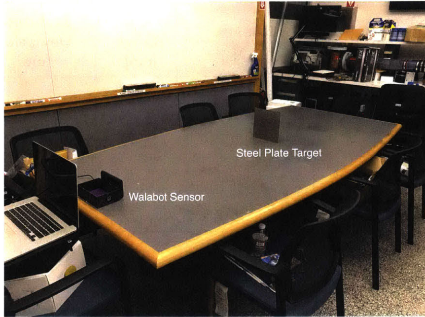
Figure 3-4: Image of test setup for radial testing
