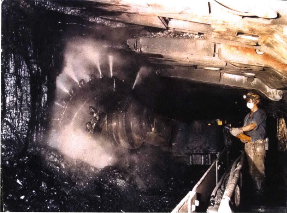
Figure 1-2: A longwall shearer with water sprayers [4]
