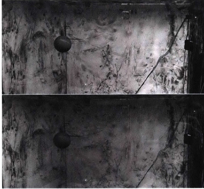
Figure 4-6: Comparison of first and last grayscale frames in 24g coal dust testing video
