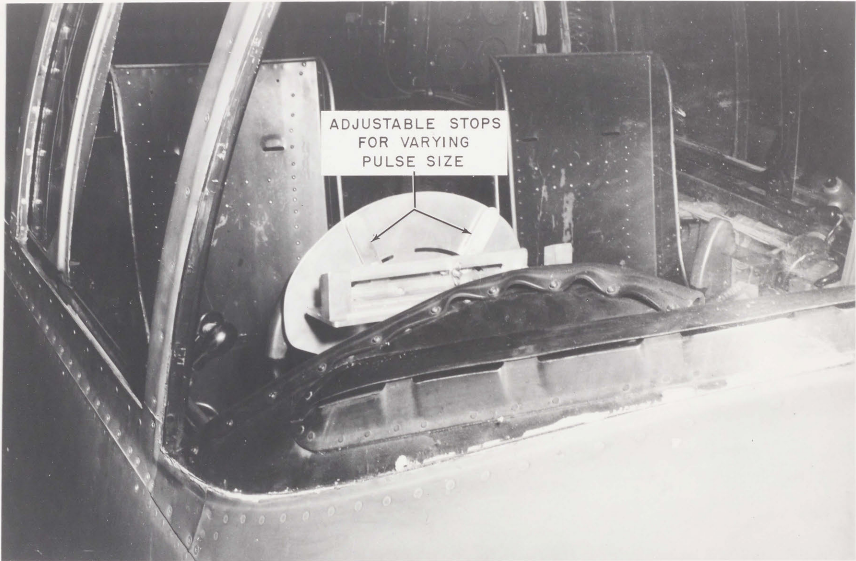
FIG. B-2. CONTROL DEVICE FOR APPLYING AILERON PULSE - VIEW LOOKING AFT INTO PILOT'S COMPARTMENT.
