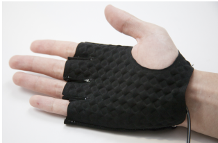
Figure 3: Haptic glove. Surface texture change of the fabric gives one a sensation of touch.
