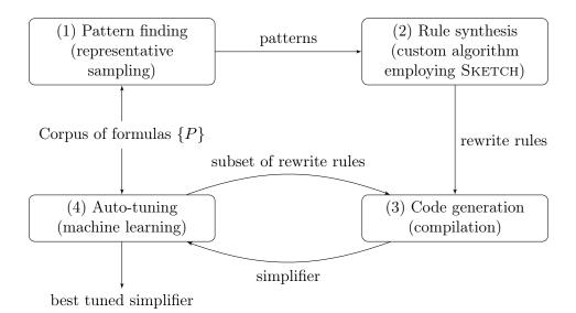
Figure 1-2: Overall phases for the SWAPPER system
