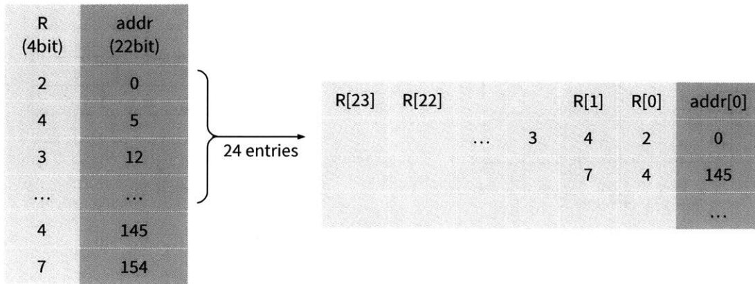
Figure 4-5: Reducing the size of Address buffer
