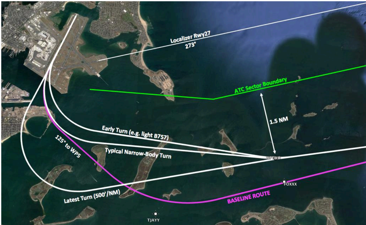
Figure 19. Procedure illustration for a 22R departure climbing via the BLZZR4 departure (baseline) compared to procedure 1-D3b
