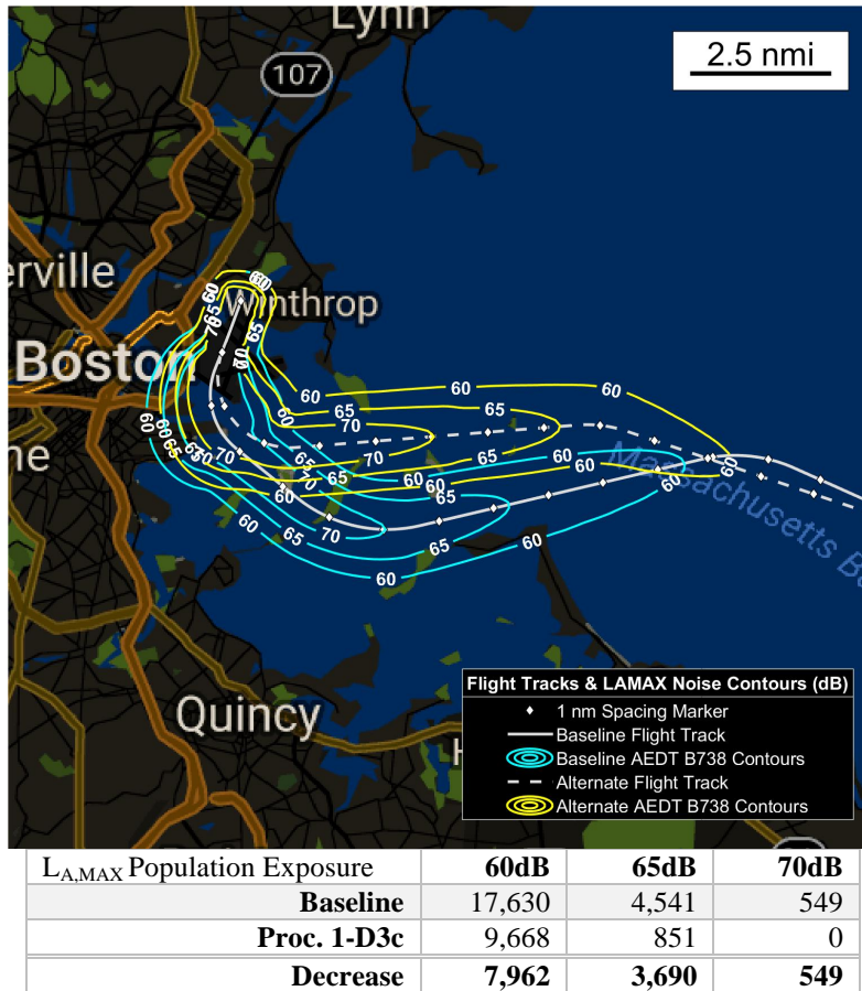
Figure 23. Noise exposure reduction for the Boeing 737-800 departing runway 22R climbing via the BLZZR4 departure on an AEDT-standard climb profile compared to procedure 1-D3c
