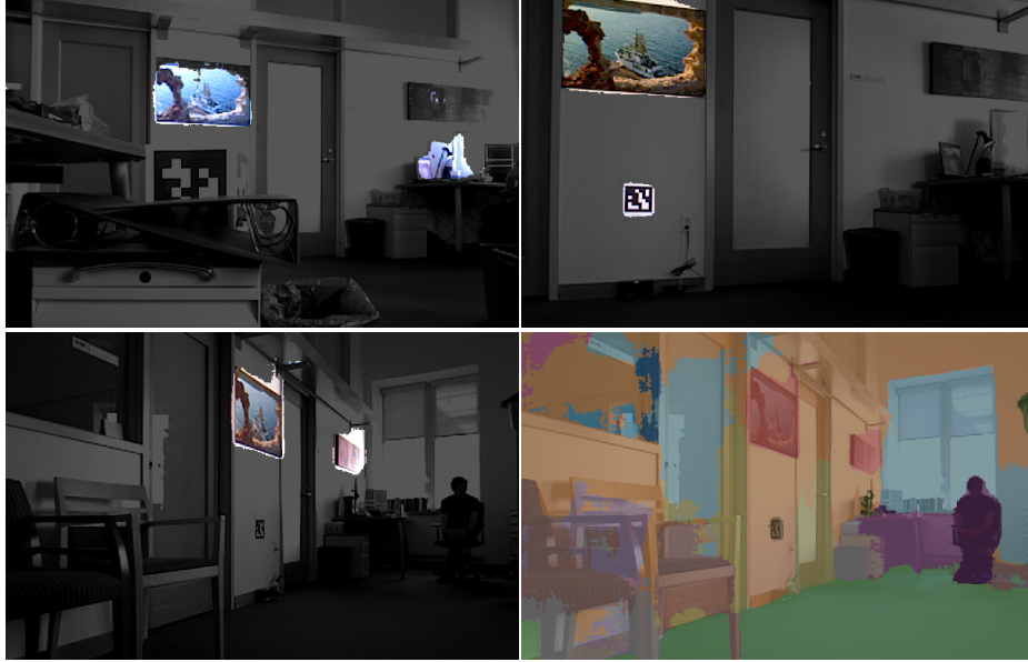
Figure 7-1: Semantic foveation with SLAM-aware backends ▶ We illustrate the potential of SLAM-aware databases that allow for semantically relevant and efficient queries in a scene. In this example, we are able to query the database for various views of the same piece of artwork that has previously been recognized. By making the database, both semantically and spatially-aware, we are able to query the semantics in a scene given its spatial location or query the different spatial locations of a given semantic entity. Furthermore, these databases can be temporally persistent that allows multi-session SLAM solutions to provide strong relational connectivity within the graph database.
