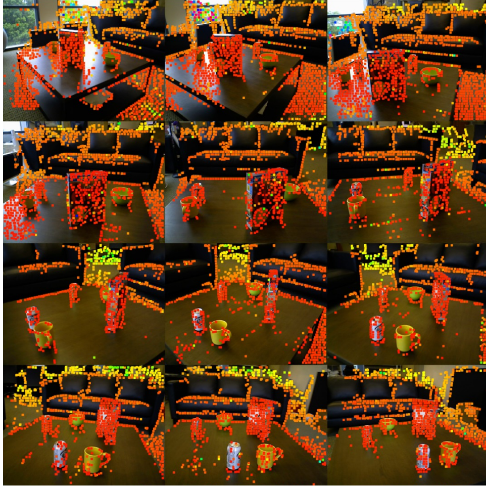
Figure 3-7: Key-frame based Multi-View Semi-dense Reconstruction ▶ Multi-view semi-dense reconstruction using keyframes significantly reduces the computational complexity of the underlying bundle adjustment (BA) problem, while simultaneously providing dense disparities and reconstructions for crucial tasks such as recovering object proposals, and reasoning about occlusions.
