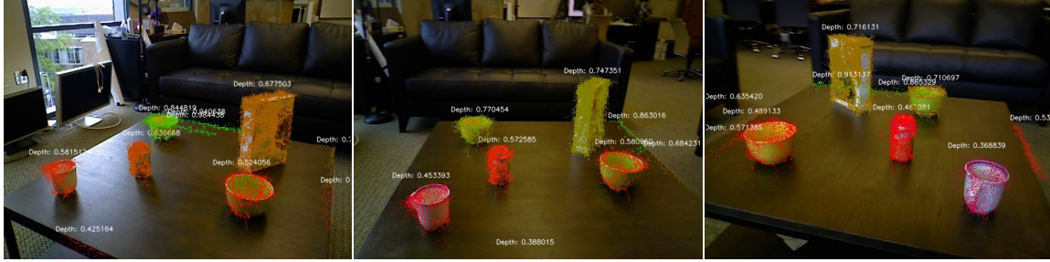
Figure 3-14: Quasi-depth estimation in scale-ambiguous maps ▶ During the object evidence aggregation step, object proposals \mathcal{O}^j \in \mathcal{O} in the reconstructed scale-ambiguous map \mathcal{M} are projected on to each of the keyframes \mathcal{K} , in order to identify objects that may be potentially occluded in that particular view. The median depths (scaled arbitrarily, but consistently across all proposals) of each object proposal is displayed in white.
