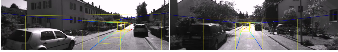
Figure 7-2: Automatic labeling for an image-based trajectory planner from hindsight experience ► By taking advantage of experience collected from human-supervised driving, we are able to project the vehicle’s future trajectory onto the current camera image, and automatically recover ground truth trajectories and their associated image for self-supervising an image-based trajectory planner.
