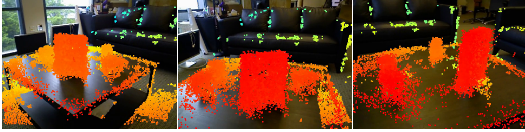
Figure 3-13: Z-buffering for occlusion handling ▶ The underlying semi-dense map reconstructed provides occlusion handling capabilities via z-buffering. This is subsequently used in the object evidence aggregation step in order to avoid mis-identifying object proposals when they are occluded by other objects.
