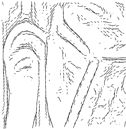
(a) The vector field obtained by fitting an oriented blurred step-function to each 3 \times 3 block of pixels (see section 4.2). The length of each vector is given by the amplitude of the brightness change normalized by the fitting error.
