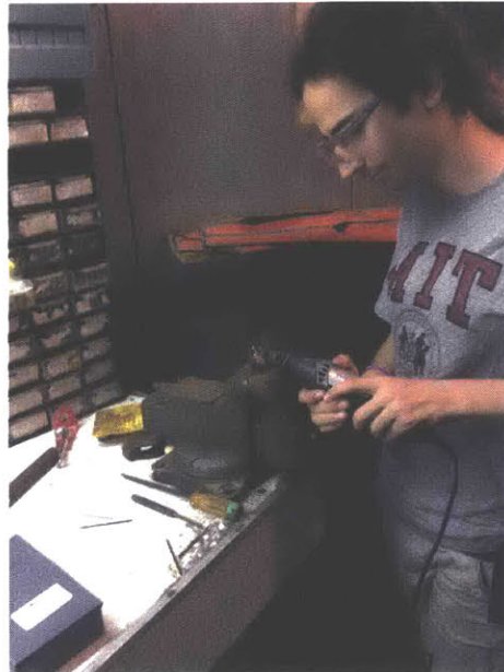
(l) 18 July 2014 - Olivia Brode-Roger milling shims to level the dome.
