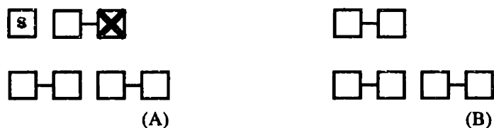
Figure 5. 13. In case of a machine failure (A) a spare machine s is used to host the repaired processes (B).
