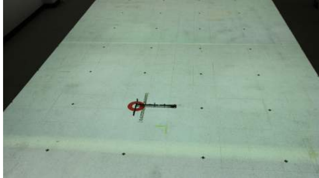
(a) Pixel space to Vicon space mapping is performed using a reference wand to map a calibration grid's vertices to motion-capture coordinates. Delaunay triangulation is then used to perform the mapping.
