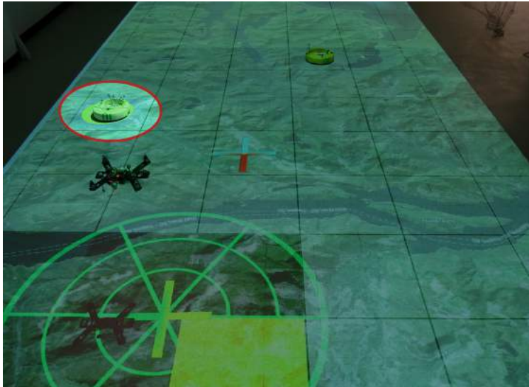
(a) A ground vehicle which has been previously detected by a surveillance quadrotor is given a highlighted color. This creates an easily-discernible contrast between detected and still-camouflaged ground vehicles.
