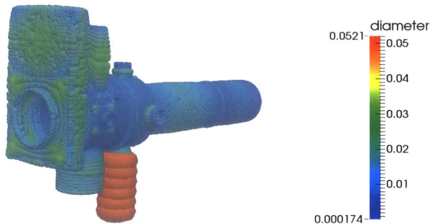
Figure 7-1: Depiction of the size and placement of the bounding balls generated from applying the pre-processing step to the KATRIN detector region mesh.
