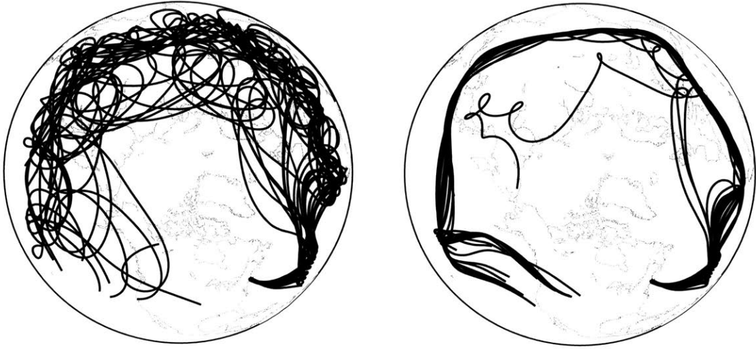
Figure 3-3: Left : Twenty five trajectories calculated with the frictionless dynamic model. Parcels were launched in an evenly-spaced 5x5 grid with its lower-left corner at 41°N, 72°W and upper-right corner at 42°N, 71°W. The large spirals are implausible for jet stream flow and reflect a problem with the model. Right : The same parcels with trajectories calculated by the dynamic model with friction. A few parcels still exhibit unrealistic spirals, but in general, trajectories are more plausible.
