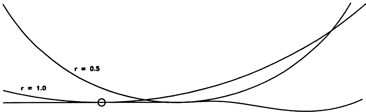
Figure 3-9: The bottom boundary of the two-dimensional region B . The radius function is approaching 0.5 as we approach the origin from the right. However, at the origin, a circle of radius 1 fits inside B , so there is a discontinuity in the radius function.
