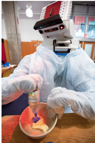
Fig. 1 BakeBot, a PR2 robot system that executes simple baking recipes. The PR2 is modified with a protective covering to prevent damage from spills and a spatula which is bolted to the end effector to enable mixing.
