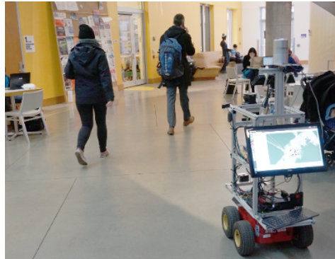
Fig. 1: A robotic vehicle navigates autonomously in a dynamic indoor environment. The vehicle uses a SICK Lidar for localization, and a Velodyne for obstacle detection.
