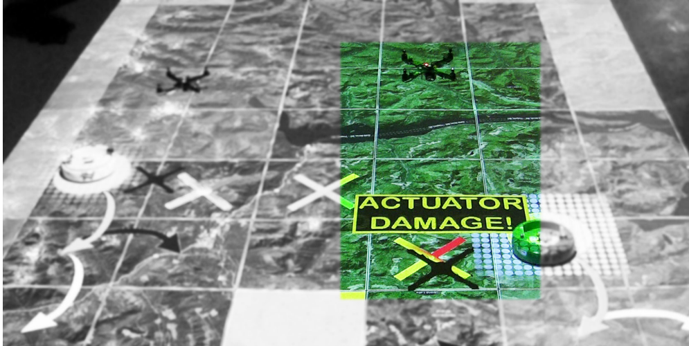
Figure 3: Vehicle health monitoring messages, such as damage of actuators or physical systems, can be displayed in real-time within MAR-CPS.
