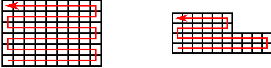
Figure 4-22: Cross section of the large MOT coil (left) and the small MOT coil (right): this shows the number of windings. The arrow shows how we wound the coil, which corresponds to the order of water flow.
