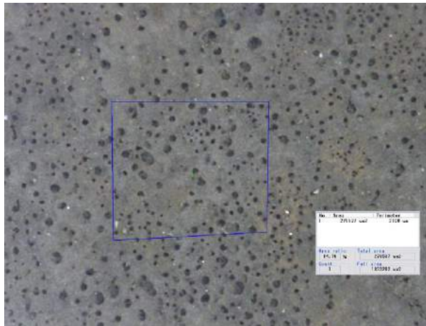
Figure 2-33: Top down view on crud formation grown in the WALT loop as shown in this figure shows its boiling chimney structure. This is obtained from technical report published by Wang on the WALT loop results in 2011 [8]. Scale bars not provided.
