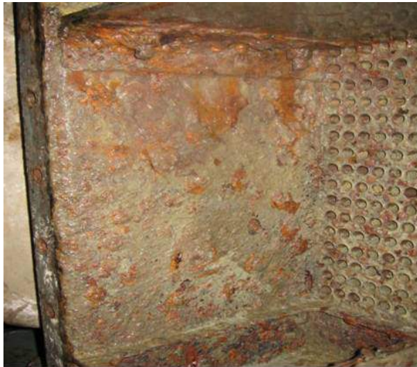
Figure 1-7: Fouling deposits in the condenser of a power plant, composed of both precipitate fouling and corrosion fouling. The dirty yellow-green layers are caused by the scaling of calcium, while the reddish layers are iron oxide corrosion products [27].
