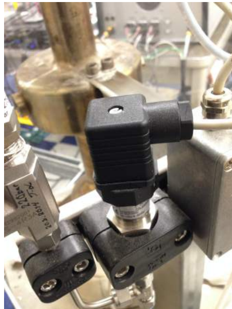
Figure 3-32: Photo of autoclave pressure transmitter.
