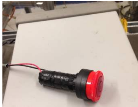
Figure 3-41: Photo of emergency switch for the heating tapes.
