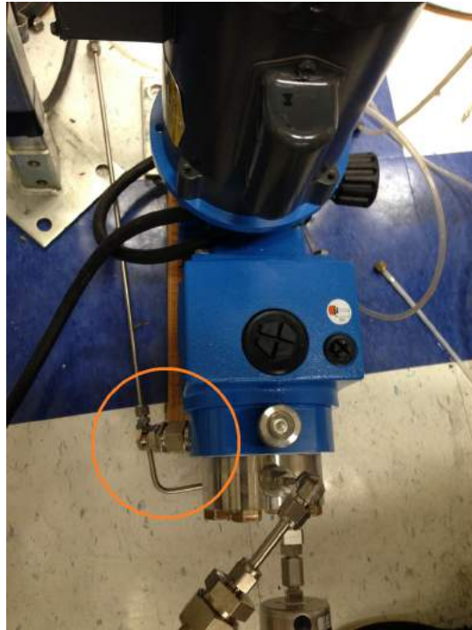
Figure 3-93: Safety valve attached to the pressurizing pump is circled in orange.
