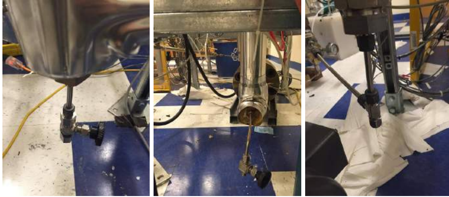
Figure 3-105: These three photos show the ports that must be opened for all the water in the loop to be drained. The first valve is the valve on the bottom of the loop near the autoclave which should drain the water from the autoclave and the tubings near it. The second valve is used to drain the circulation pump and the tubings near it. The cap is used to drain the water near the pressurizing pump.
