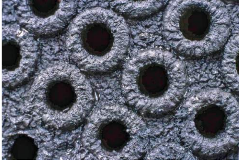
Figure 1-2: This image shows the asphaltenes fouling on the heat transfer surface of a heat exchanger in a crude oil refinery. This is a common type of chemical fouling [16].
