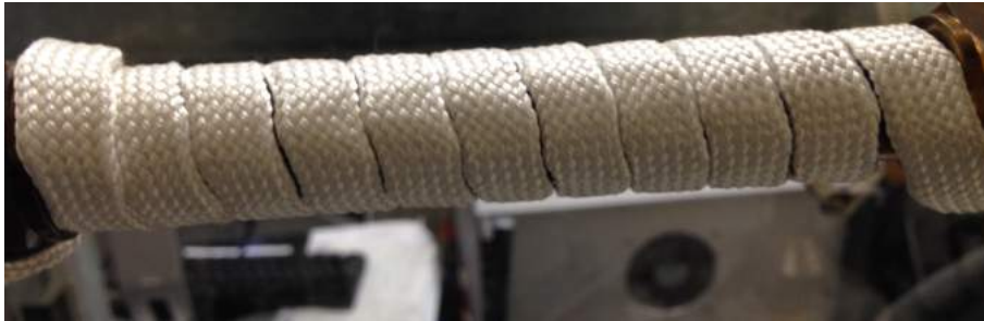
Figure 3-37: This heating tape becomes white and brittle after several experimental runs.
