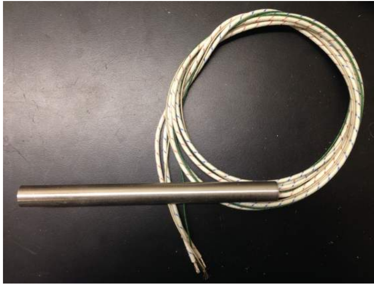
Figure 3-28: Photo of heating cartridge before being press-fitted inside an autoclave heater rod.
