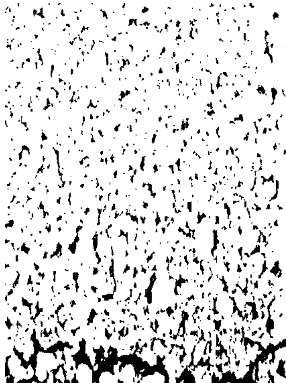
Figure 5-22: Binary image converted from the cropped image in figure 5-20 using Otsu thresholding. This image is used to obtain the porosity and the fractal dimension.
