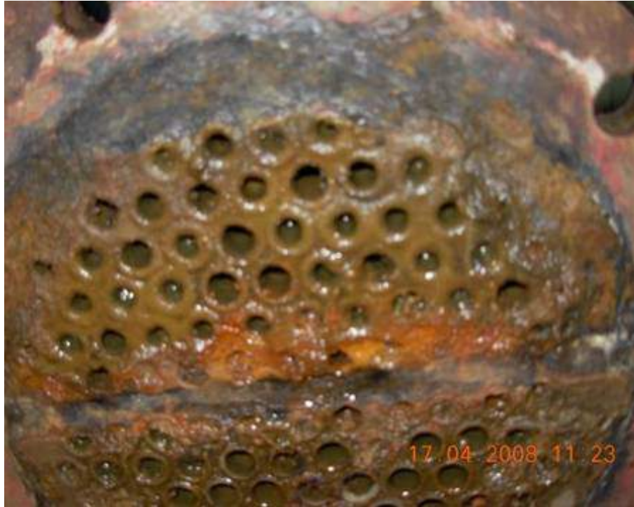
Figure 2-9: This image shows foulings on an industrial heat exchanger. It is a combination of both lime scale precipitation fouling as well as an algae biofouling [68].
