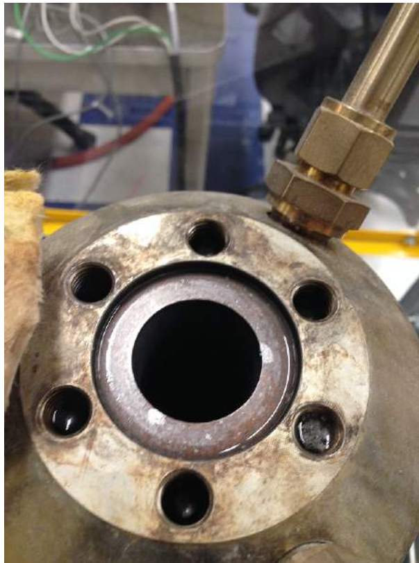
Figure 3-99: Photo of the autoclave's top opening where the top flange can be inserted.
