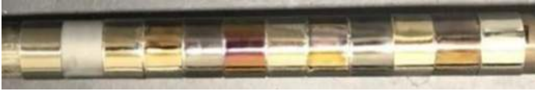
Figure 3-10: Sample rings covering the heater rod. Sample rings are where we grow crud. Different ring colors are due to different types of coatings applied. From right to left, the samples are coated with 316 stainless steel, ZrC , ZrN , TiC , TiN , Al_2O_3 , TiO_2 , TiB_2 , ZrO_2 , MgO , Ti_2AlC , and zircaloy, respectively.
