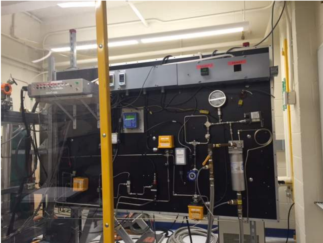
Figure 3-61: This is the photo of the auxiliary loop. The auxiliary loop is used to measure and regulate the loop chemistry.
