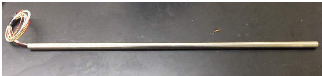
Figure 3-27: Photo of an autoclave heater rod with heating cartridge press-fitted inside.
