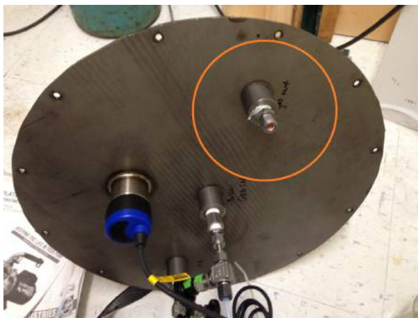
Figure 3-97: Top lid of the water tank. The chemical injection port is circled in orange.
