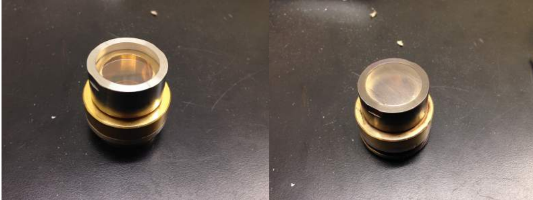
Figure 3-106: A new autoclave window (left) versus a used, corroded autoclave window (right).
