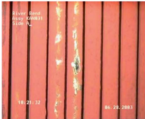
Figure 1-11: Example of fuel rod failure caused by crud-induced localized corrosion (CILC) in the River Bend BWR [42]. At the end of cycle 11 at River Bend, six failed fuel assemblies were identified. The hole in the middle fuel rod in the image is one of the fuel failures. The orange coverings around the fuel rods are crud.
