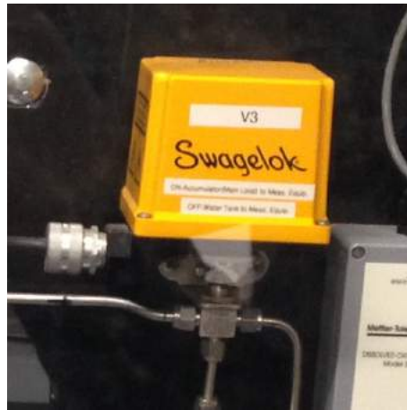
Figure 3-71: Photo of valve and its actuator. The valve is the part attached to tubings while the actuator is the yellow box.
