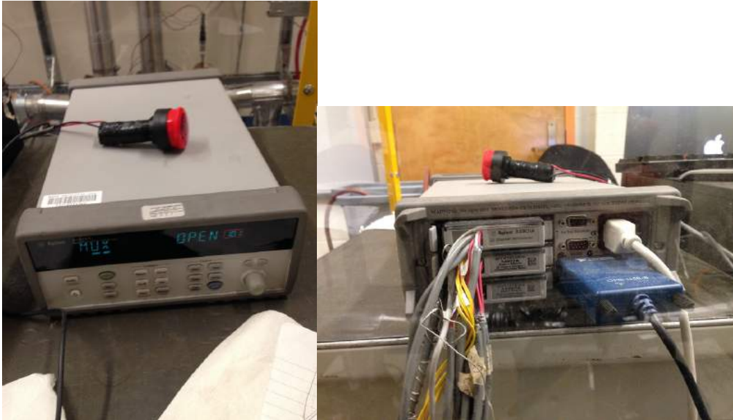
Figure 3-84: Photo of Agilent data acquisition and control unit's frontside (left) and backside (right).
