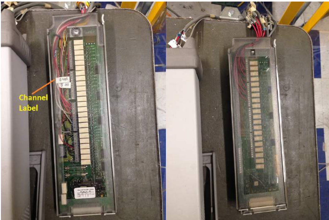
Figure 3-85: Photo of Agilent data acquisition board (left) and relay board (right). Each wire is labeled with the channel it connects to. More information on wiring can be found in subsection 3.7.2.5.
