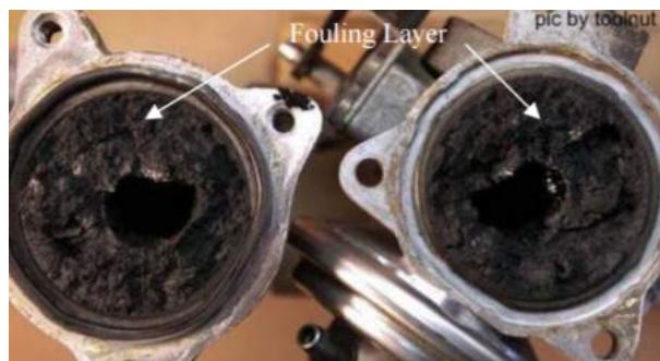
Figure 2-1: This image shows particulate fouling in the Exhaust Gas Recirculation (EGR) cooler in a diesel engine. [57].
