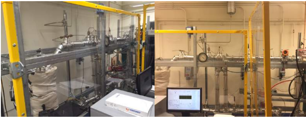
Figure 3-24: This figure shows the photos of the main loop from different angles. Notice the autoclave on the left of both pictures wrapped in the heat insulators. This autoclave is where the experiment is carried out.
