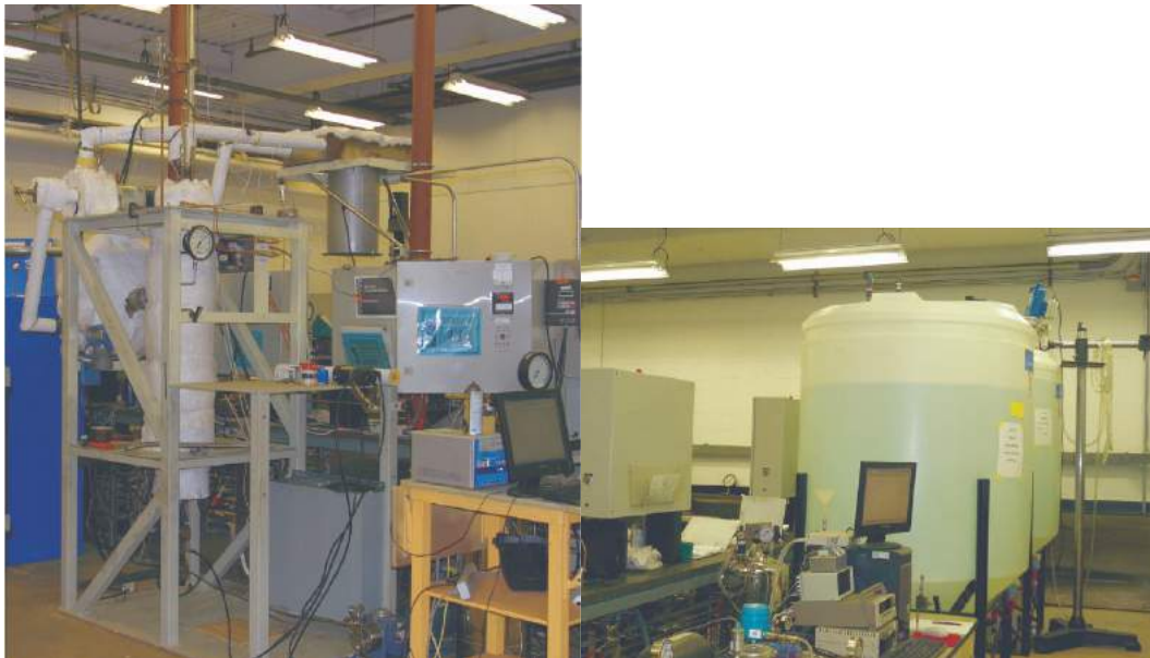
Figure 2-58: The left photo shows the WALT loop's autoclave setup where the test section is located and the actual crud growth occurs. The right photo is the photo of the WALT loop's chemical control system [8].
