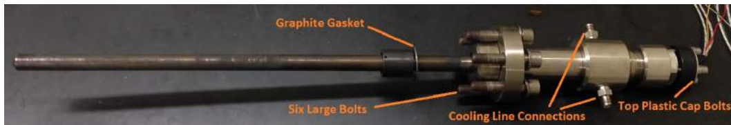
Figure 3-98: Photo of top flange heating rod assembly. Each component mentioned in the insertion instruction is labeled.
