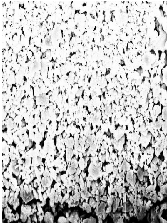
Figure 5-20: Cropped cross-section view SEM image of crud obtained from cropping figure 5-19.
