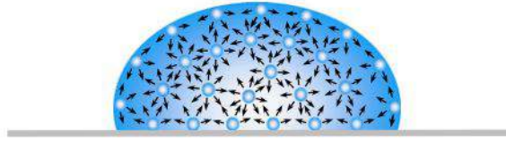
Figure 6-15: Illustration of the dynamics within the water droplet sitting on a surface. Circles are the liquid molecules which pull each other together by the force shown by the arrow [230].
