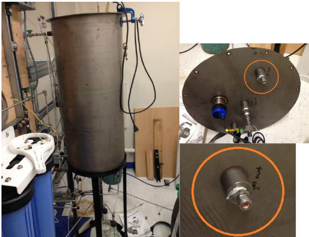
Figure 3-78: The water tank photo (left), the water tank lid photo with the chemical injection port circled (top right), and the zoomed in chemical injection port.
