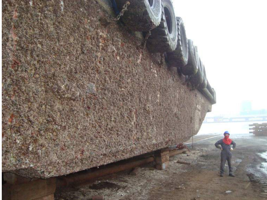
Figure 2-8: This image shows a ship hull covered with a biofouling layer [67].
