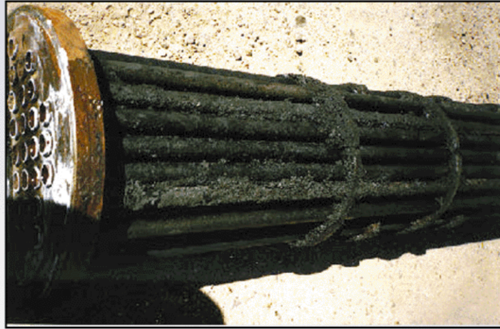
Figure 2-7: The condenser tubing shown in this image is covered in solidification foulings partially caused by solidified hydrocarbon [65].
