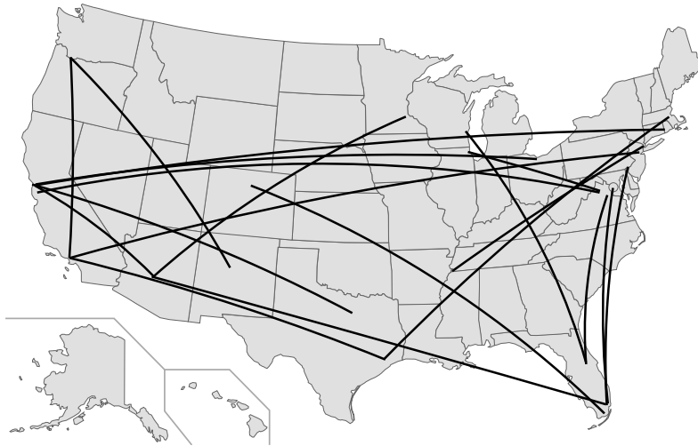
Figure 3. Illustrated here are the 20 representative flight trajectories flown by the Boeing 737-800W in the TASOpt-AEDT uncertainty quantification study.
