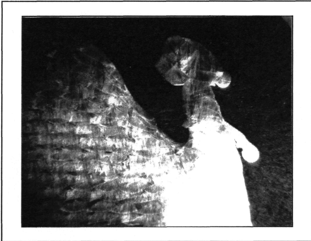
FIGURE 4.17 Multilayer Defect in 308 SS EB Deposit, 10X
