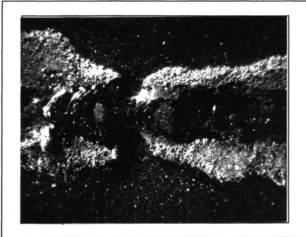
FIGURE 3.22 Unreacted powders Spot-Welded onto Steel Sheet, 12 X Material C Precursor, Single EB Melt Pattern is Visible, EB Assisted Reaction Synthesis
