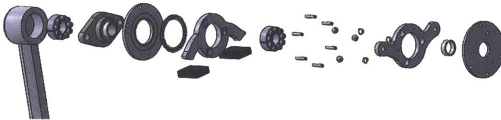
**Figure 16:** Lower enclosure, full assembly, screws missing.
