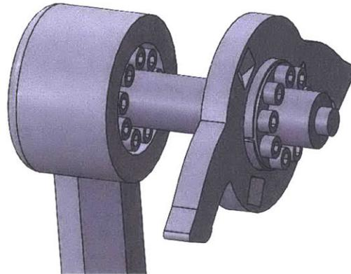
**Figure 12:** Handle attachment with keyless bushings
