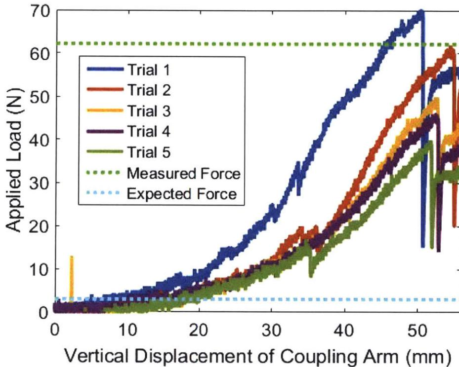
**Figure 21:** Input load (N) on the coupling arm as it is displaced. Average measured overload force is 62.2 N, twenty times higher than expected.
