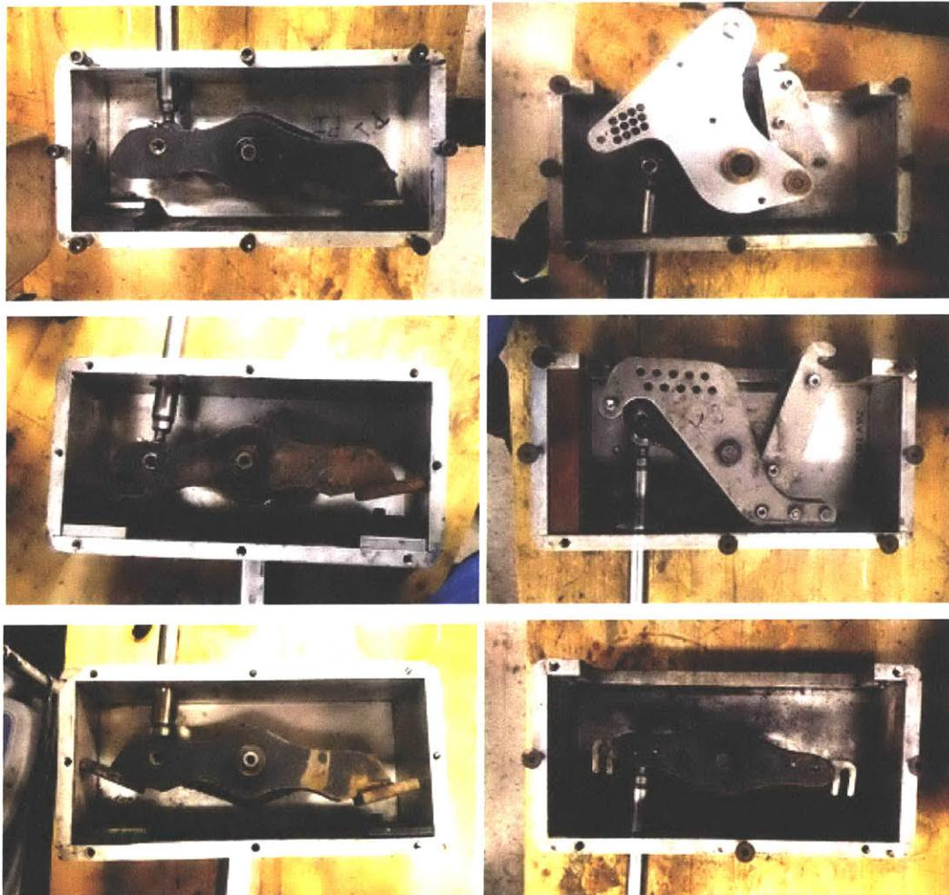
**Figure 3:** Current actuation systems for Pythagoras (top), Kepler (middle), and Galileo (bottom). Lower mechanisms on the left, upper mechanisms on the right.
