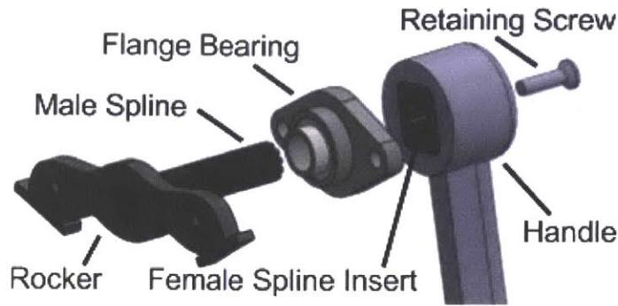
**Figure 4:** Exploded view of the handle attachment within the current system, lower enclosure omitted.
