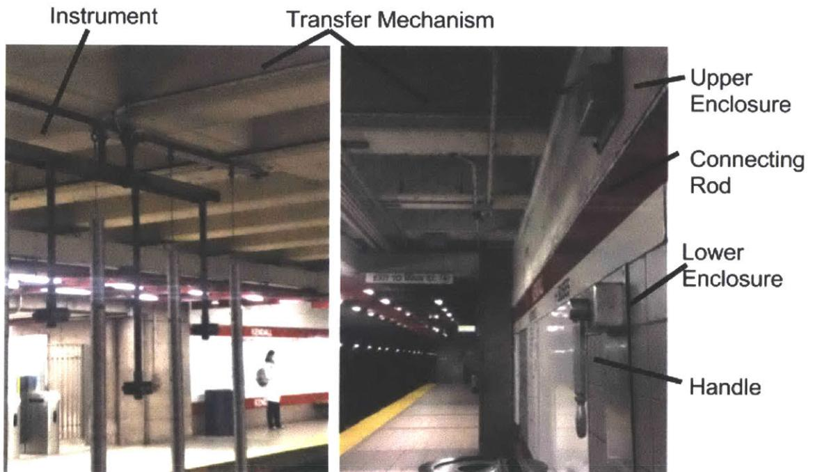
**Figure 2:** Kendall Band instrument architecture-- handle, platform enclosures, connecting rod (missing), transfer mechanism, and instrument.
