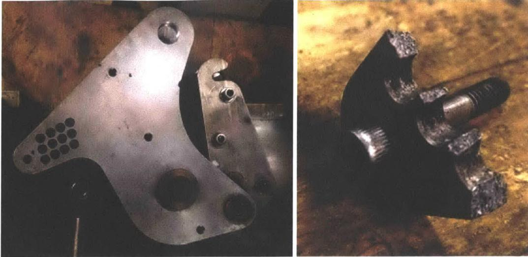
**Figure 10:** Upper-enclosure mechanism for Pythagoras (left; missing: retaining rods) and a fragment of its exterior plate (right).
