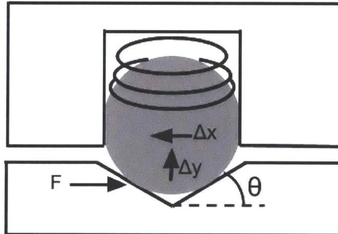
**Figure 18:** Diagram of the ball and groove displacement
