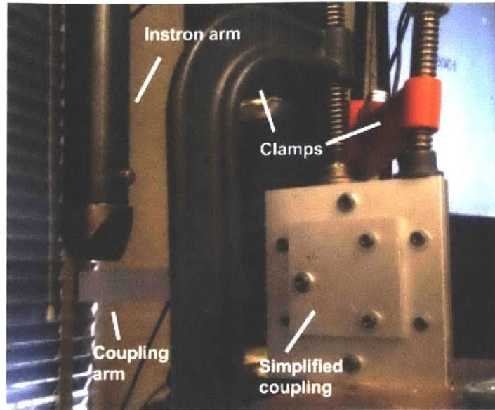
**Figure 20:** The stress relief test apparatus, including the simplified coupling, and the Instron testing system
