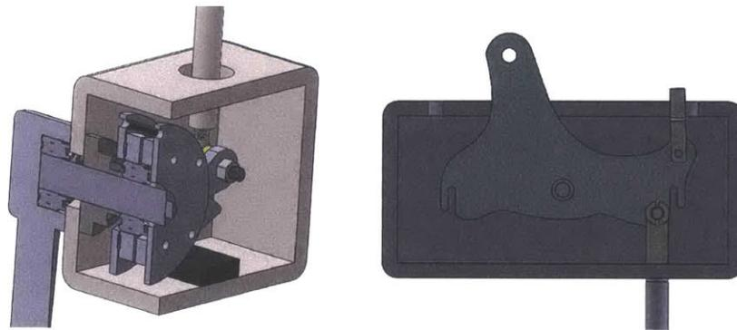
**Figure 11:** New actuation system, lower (left, split view) and upper (right) assemblies
