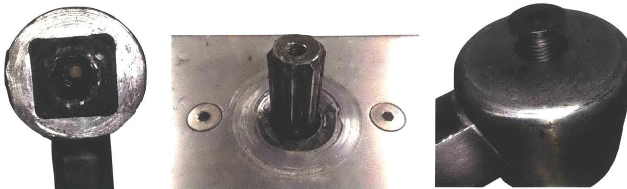
**Figure 9:** Female spline coupling within handle (left), male spline coupling protruding from lower enclosure (center), retaining screw for handle (right). Wear can be seen upon the female and male halves of the coupling.
