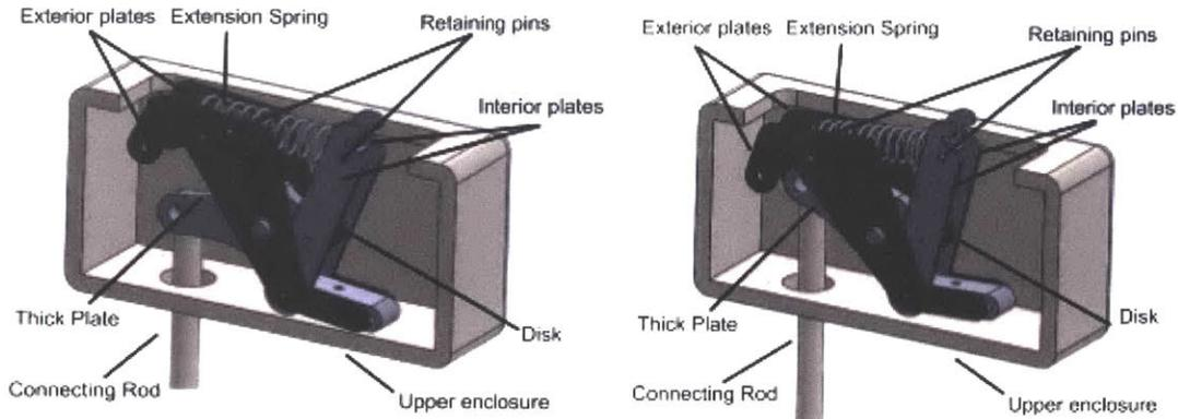
**Figure 6:** Kepler's upper mechanism, disengaged (left) and engaged (right).
