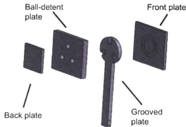
**Figure 19:** Simplified coupling assembly (fasteners, springs, and balls omitted)
