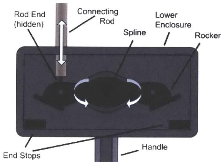
**Figure 5:** Motion and components within the lower enclosure.
