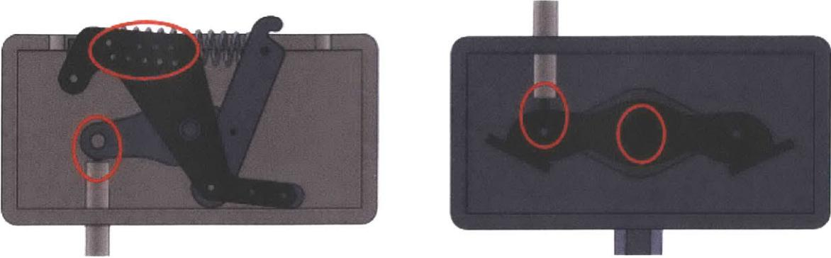
**Figure 8:** Failure points within the current actuation system, circled in red.
