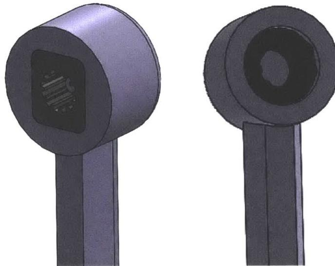
**Figure 13:** Current handle with spline insert (left); Modified handle with bushing (right).
