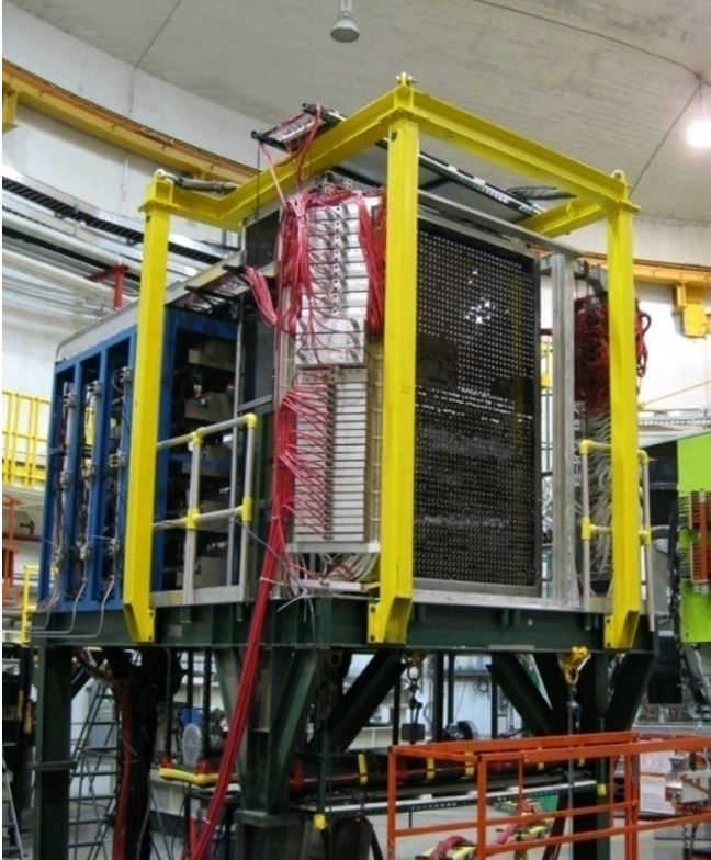
FIG. 5. BigCal calorimeter with its front aluminum shielding plates removed, exposing the stack of 1744 lead-glass blocks.
