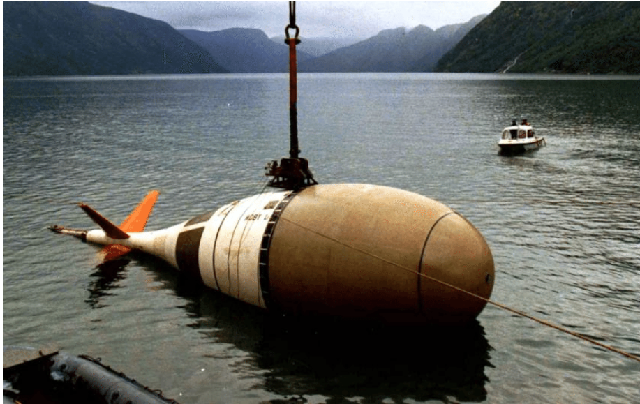
Figure 1-2: The Admiralty Research Establishment's (ARE) high speed buoyancy propelled vehicle called MOBY-D used for testing the effect of riblets on drag reduction. This vehicle is 12.6 m long and 3.35 m in diameter [8, 9, 10].
