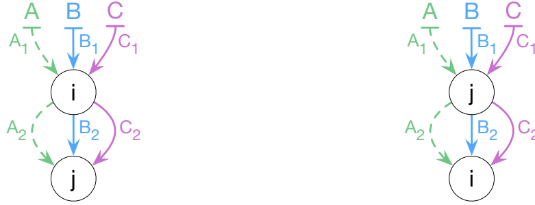
(a) Iteration graph for CSR matrix addition (b) Iteration graph for CSC matrix addition
