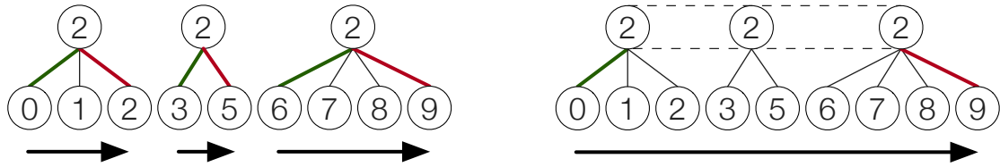
(a) Each coordinate position iterator iterates over the children of a duplicate coordinate.
