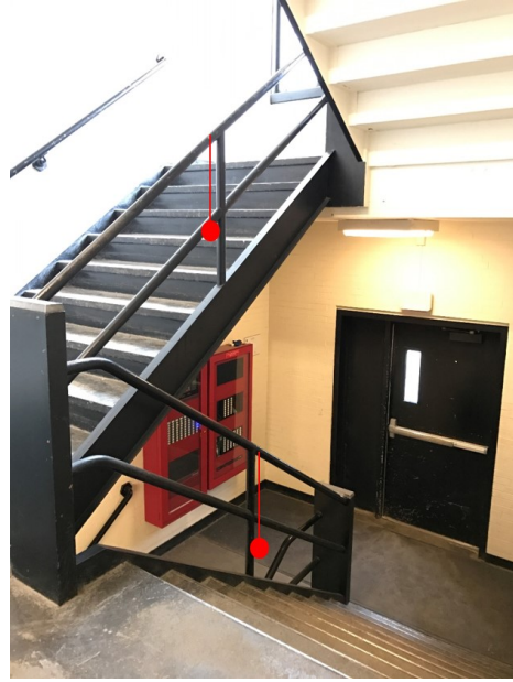
Figure 3-6: Locations of the thermometers when hanging from the railings. Red dots represent thermometers.
