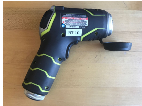
Figure 3-7: The infrared thermometer measuring surface temperatures in the experiment.
