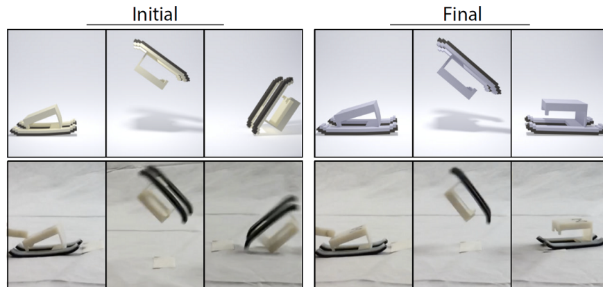
Figure 4-21: A comparison of experimental (bottom) and DAC/BBI simulated (top) results for initial (left) and final (right) designs of a flipping mechanism.
