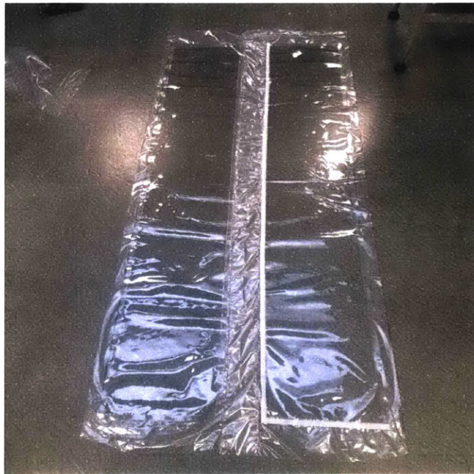
Figure 7 Top of enclosure made with vinyl and LDPE with airflow tube in the middle
