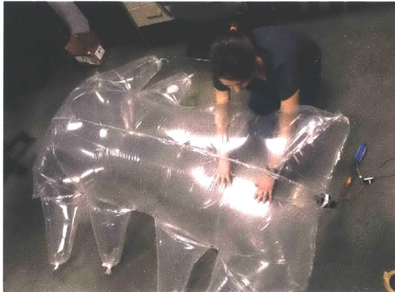
Figure 13 Demonstrating a first prototype of an inflated enclosure. Method of fabrication: sewing
