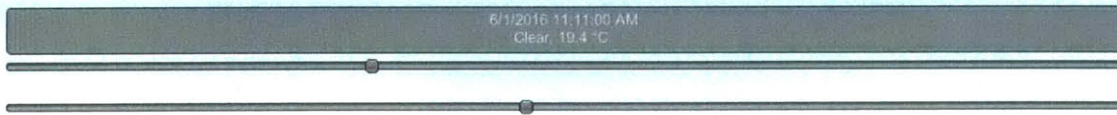
Figure 5-2: Doppelmarsh's Timeline UI features two sliders. The first is used to change the day since October 2014 until the present moment, whereas the second is used to specify the time of the day.
