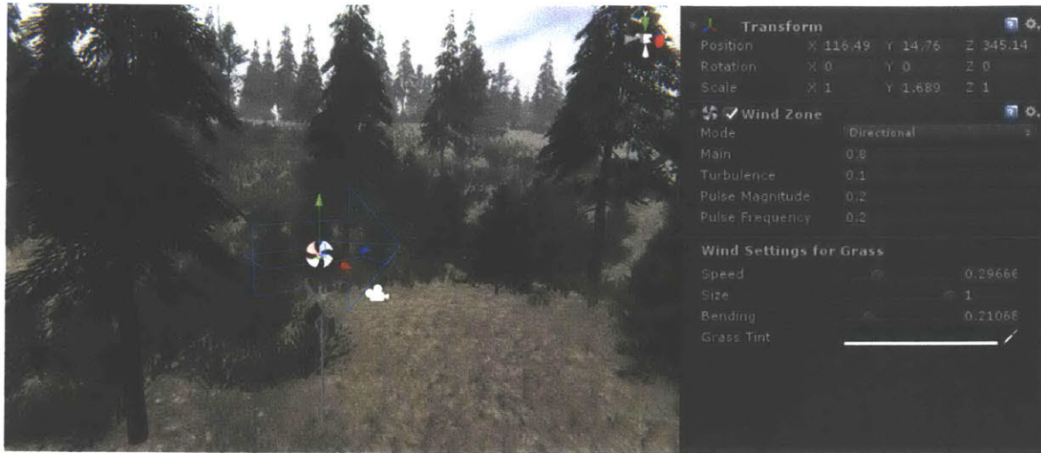
Figure 4-5: Two main wind-zones in governs Doppelpmarsh. The first is responsible for simulating the wind's effect on trees and objects, and the second controls the wind's effect on the grass. The reason to this redundancy is because the grass in Unity is rendered as a texture, whereas the trees are rendered as a mesh model.
