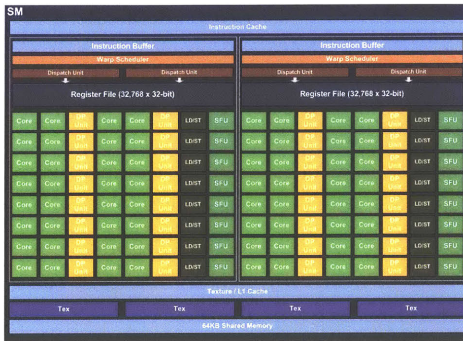
Figure 2-16: SM configuration of the NVIDIA Pascal GP100 GPU [34].
