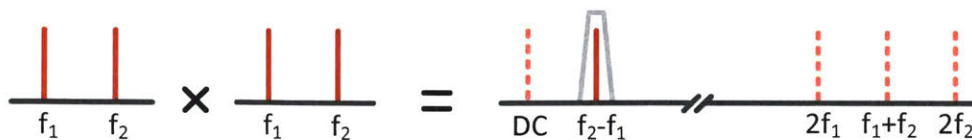
Figure 2-1: Illustration of AirShare’s Design. Wireless nodes multiply the received signal by itself and extract the desired clock signal by applying a band pass filter centered at f_{ref} .
