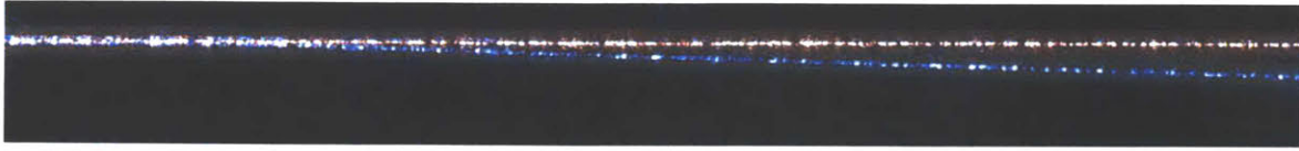
Figure 5-19: Colored and overlaid infrared images of the dichroic filter operation. Blue: \lambda_1 = 1530 \text{ nm} < \lambda_C , Red: \lambda_2 = 1535 \text{ nm} > \lambda_C
