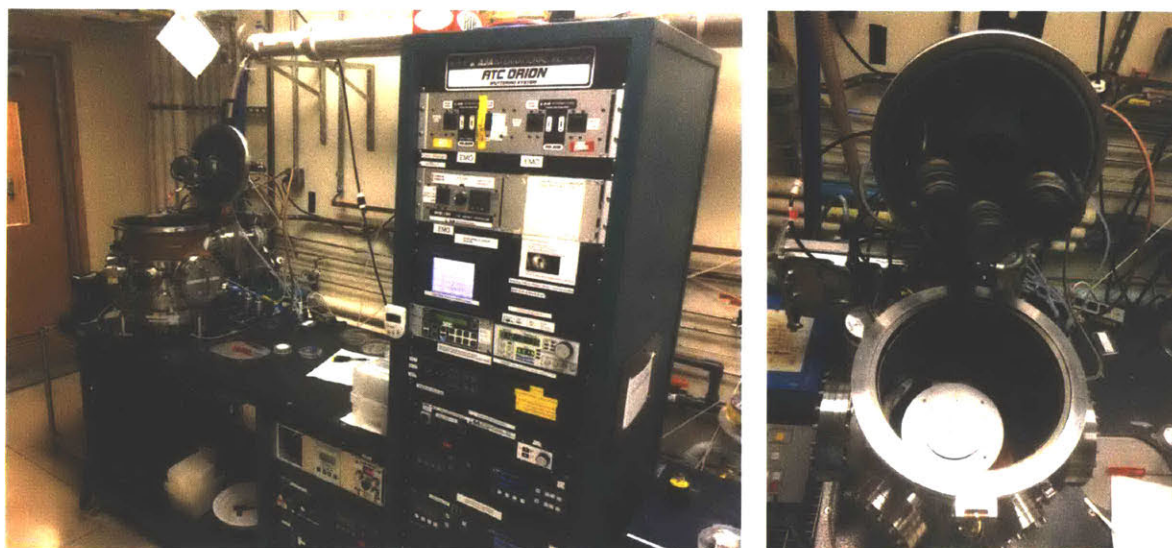
Figure 3-1: A photograph of the AJA Orion sputtering tool located in EML of Microsystems Technology Laboratories at MIT, and a close-up view of the sputtering chamber with upside-down magnetron guns on the cover
