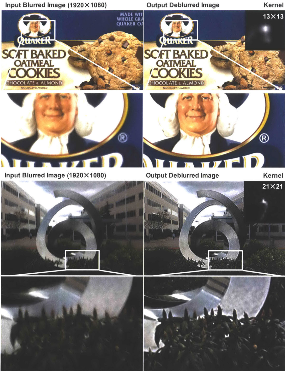
Figure 2-16: Test 1920 × 1080 blurred image, output kernel of size 13 × 13 (top) and 21 × 21 (bottom) and deblurred image.
