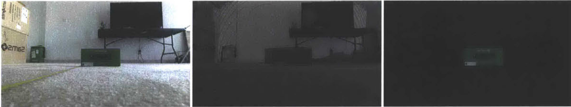
Figure 4-10: Area measurement of a box with a known surface area at 914 mm (approximately 3 ft). The image taken with a Kinect V2. A ruler on the floor measures the true distance of the box. Left: The color image. Middle: The color image overlaid with the mapped depth image. Right: Segmentation result.
