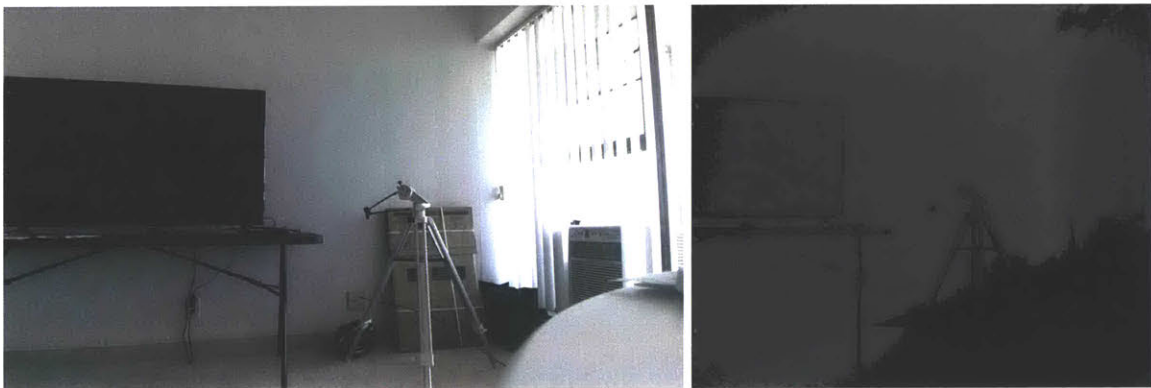
Figure 4-3: Images captured by Kinect V2: Left: Color image ( 1920 \times 1080 ), Right: Depth image ( 512 \times 424 ). Dimensions of the two images are different. Black area indicates missing depth values.
