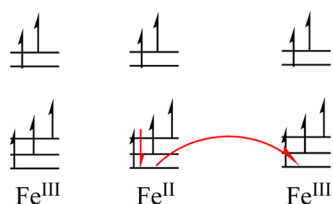
Figure 17. Simplified diagram illustrating how the extra electron associated with the Fe II center in magnetite can delocalize when all of the unpaired spins are aligned. If neighboring Fe III centers were aligned antiparallel, the transfer would violate the Pauli principle.
