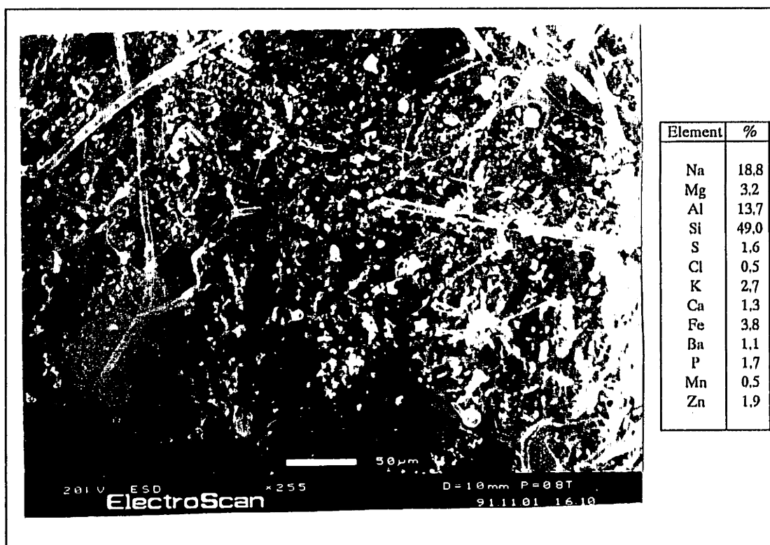
Figure III.E-8: Filter Sample Collected at Wedge Pond After a Storm Event, August 20, 1991
