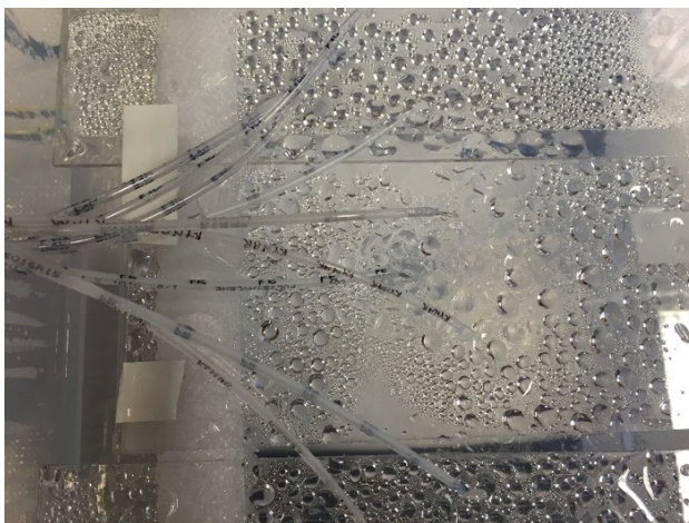
Tubes inside the high RH setup (condensation droplets on the wall due to high RH)
