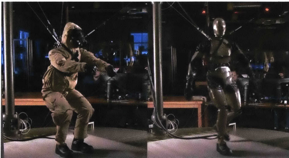
Figure 2-15. Boston Dynamic's Petman humanoid robot designed to wear and test chemical protection clothing under realistic conditions.
