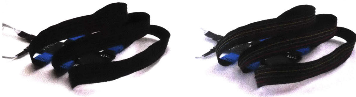
Figure 6-6. Prototype printed circuit board and thermochromic ribbon showing the all black off state (left) and the full color all on state (right).
