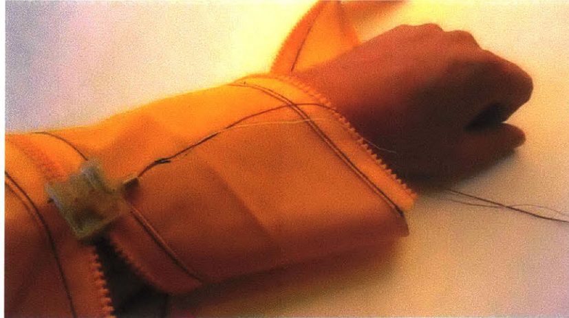
Figure 7-7. Zipperbot joining a spiral pattern piece to assemble a tube sleeve.
