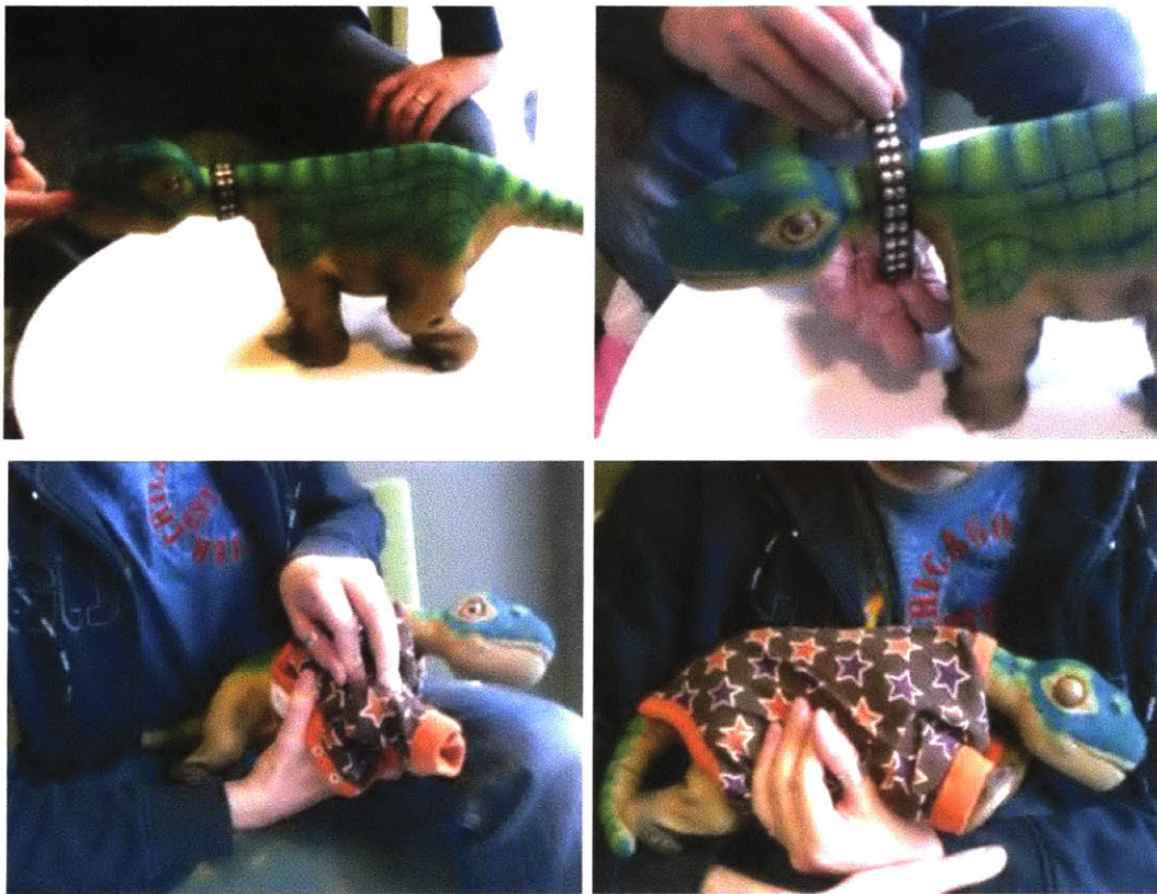
Figure 2-12. ActDresses by Feraeus and Jacobsson from the Swedish Institute of Computer Science is a design concept that uses the metaphor of clothing to control robotic devices.
