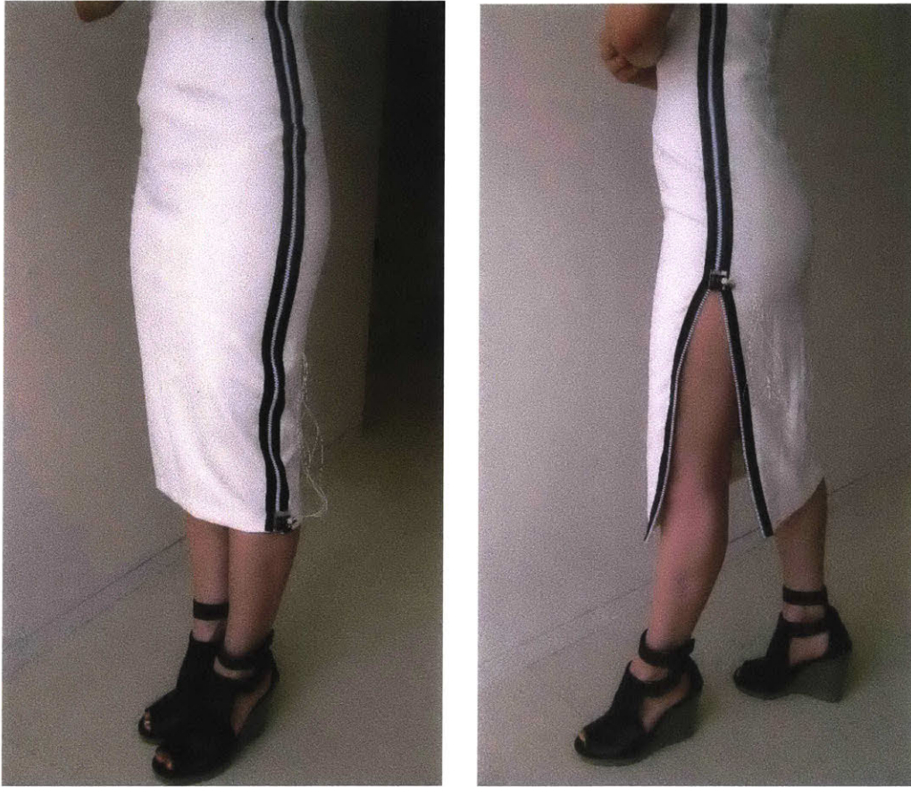
Figure 7-13. Zipperbot integrated in a hobble dress and controlled via an Android mobile device.
