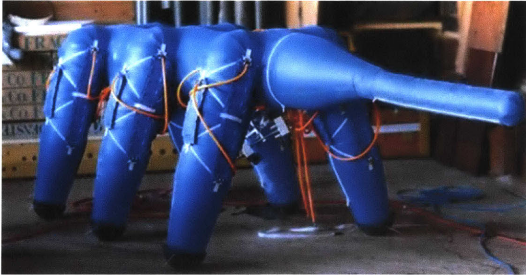
Figure 2-10. Otherlab’s low-cost, pneumatically controlled, inflatable robot, Ant-Roach .
